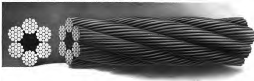
Regular lay, right hand rope, 6 x 19
