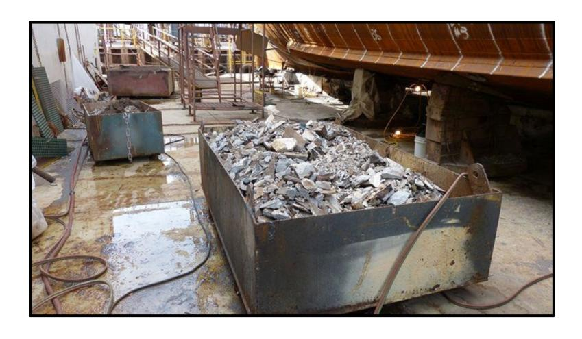
One of the many hoppers loaded with concrete removed from the bilge.
