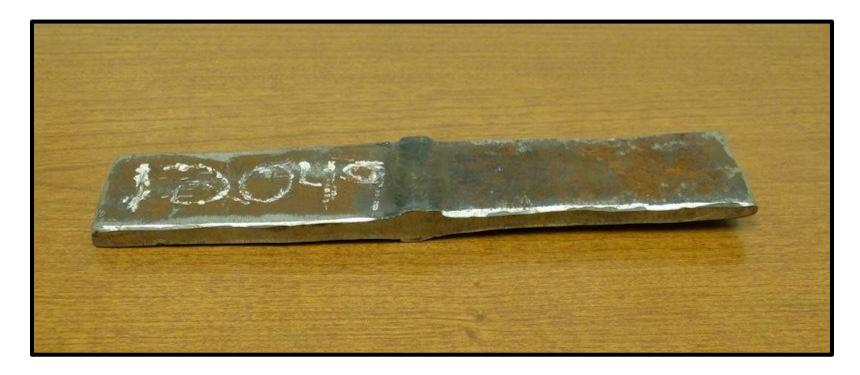
A certified shipyard welder was further required to weld up a test coupon to ensure they could safely join modern steel to 135 year old wrought iron.
