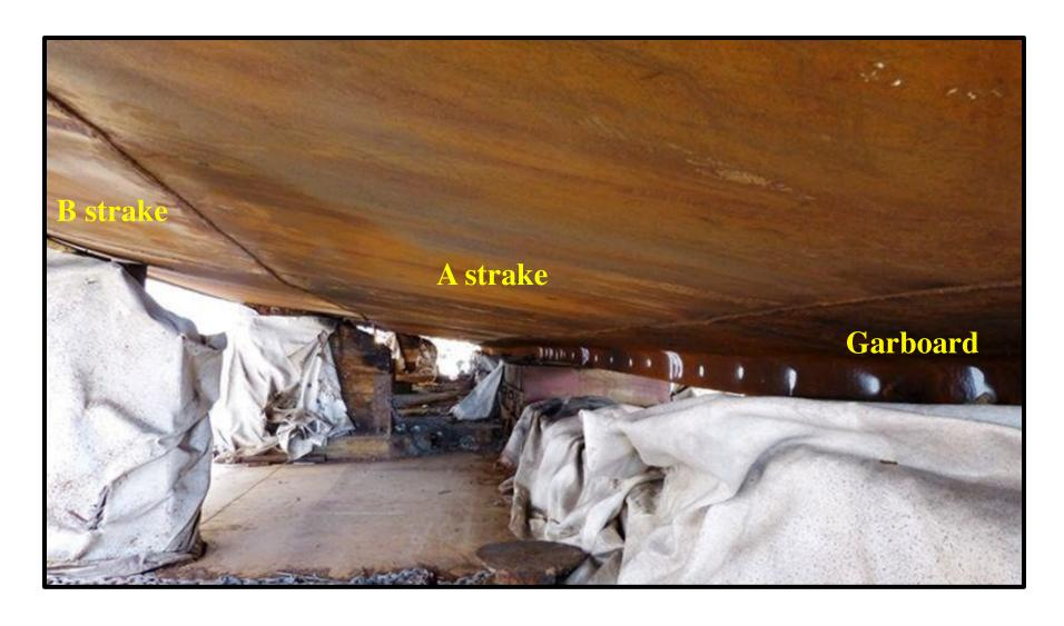
A & B strake renewed in 1/2" A-30 mild steel plate from stem to stern
