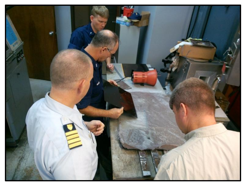
Inspecting x-rays of test plate section that was cropped out at the beginning of project.
