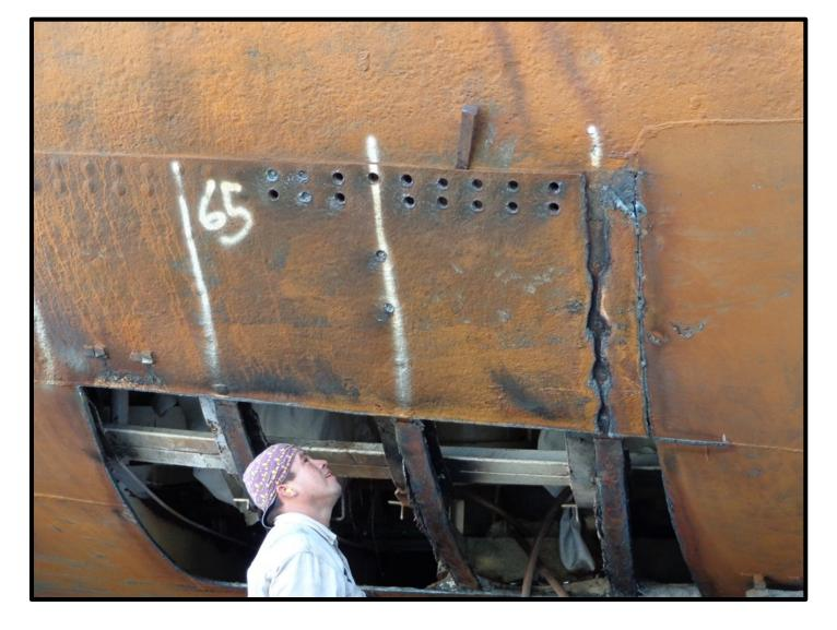
Washing off rivets and burning through hull plate. The wedges assisted in prying back the plate enough to knock out the rivet heads. This was done to facilitate a welded to rivet transition.
