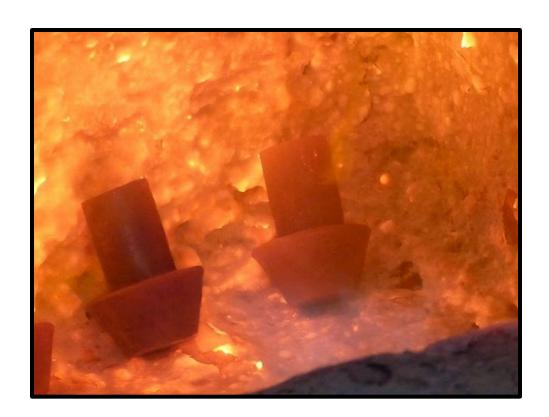
Rivets being brought to an orange heat – too hot and they burn; too cold and they do not peen over properly.
