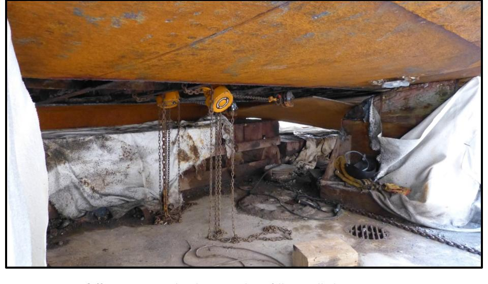
Offering up new plate by using chain falls to pull plate into position for mark up and fit up.
