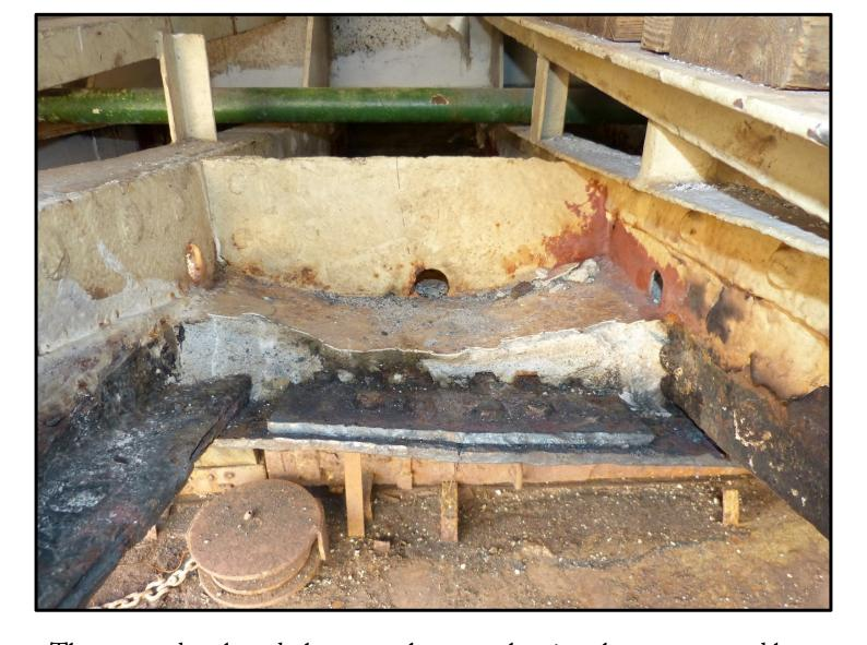
The cropped garboard plate near the stern showing the concrete and butt plate, and wash plates with limber holes in the frames. Note the shaping of the concrete to direct water to the limber holes.
