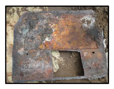
Inboard side of cut out test panel placed on the dry dock floor. This section was later radiographed after the composition test.
