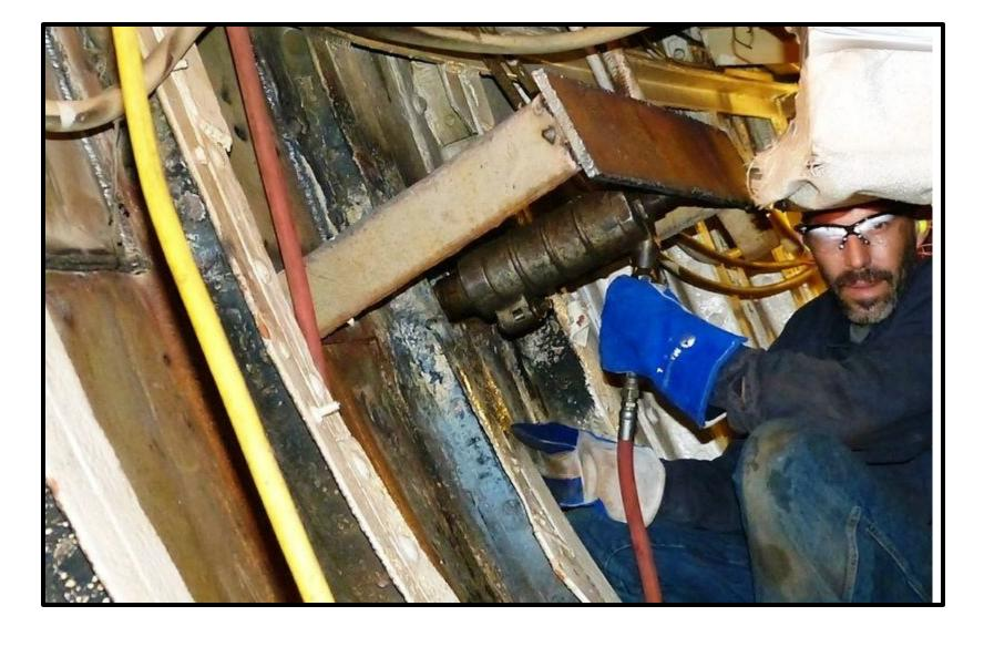
Inside the hull, a "bucking" hydraulic jack is used to hold the rivet head while the rivet point is worked outside.
