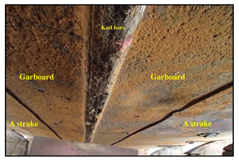
ELISSA's keel is 3 iron bars sandwiched between the port & starboard garboard plating and then through riveted together.
