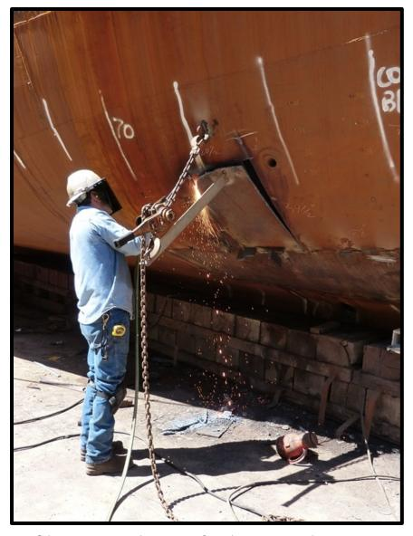
Shaping a plate to fit the complex curves of the hull.
