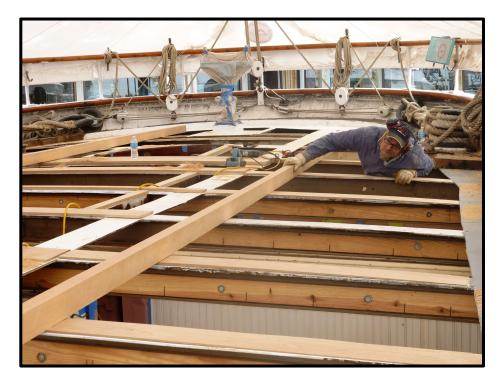
Checking the fit of the shims and decking.
