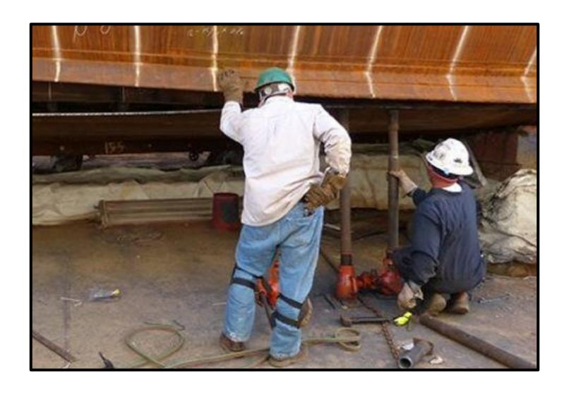
30 ton hydraulic jacks pushing plate against frames for a tight fit.
