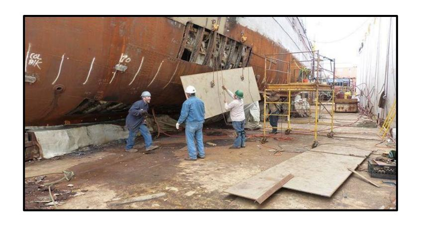
Fitting new steel plate in preparation for drilling, reaming out, and riveting.
