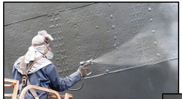
Applying the ceramic coating. It was below 50° outside, but the hull heated up to 60° with the 150° coating.
