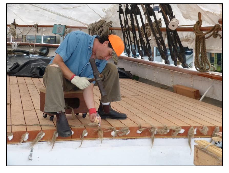
Caulking the deck with one pass of cotton and two of oakum.
