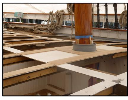
To avoid letting in the decking to lay flat against proud deck beams, all the low beams were shimed up with white oak shims. This eliminated the many cuts and exposed end grain of letting in the planks.
