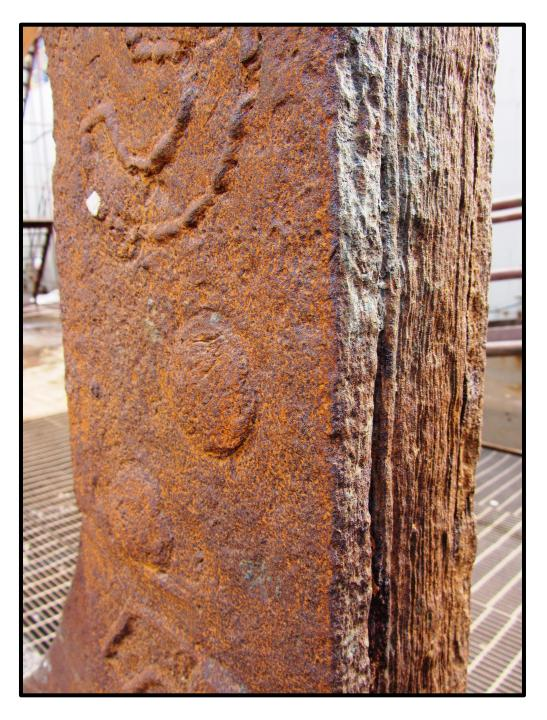
Stern post and propeller aperture.
