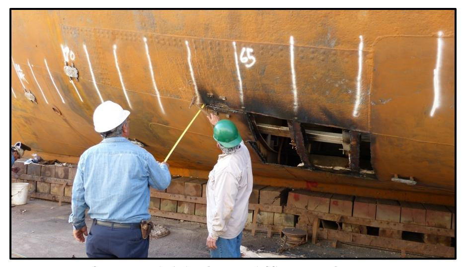
Cropping out bad plate for renewal. This cut is at frame 63 - 66 port side. Frames are numbered forward from the stern post.
