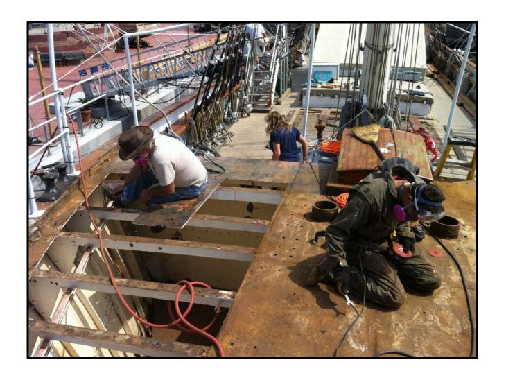
Dressing the steel plate on foc's'le head deck.
