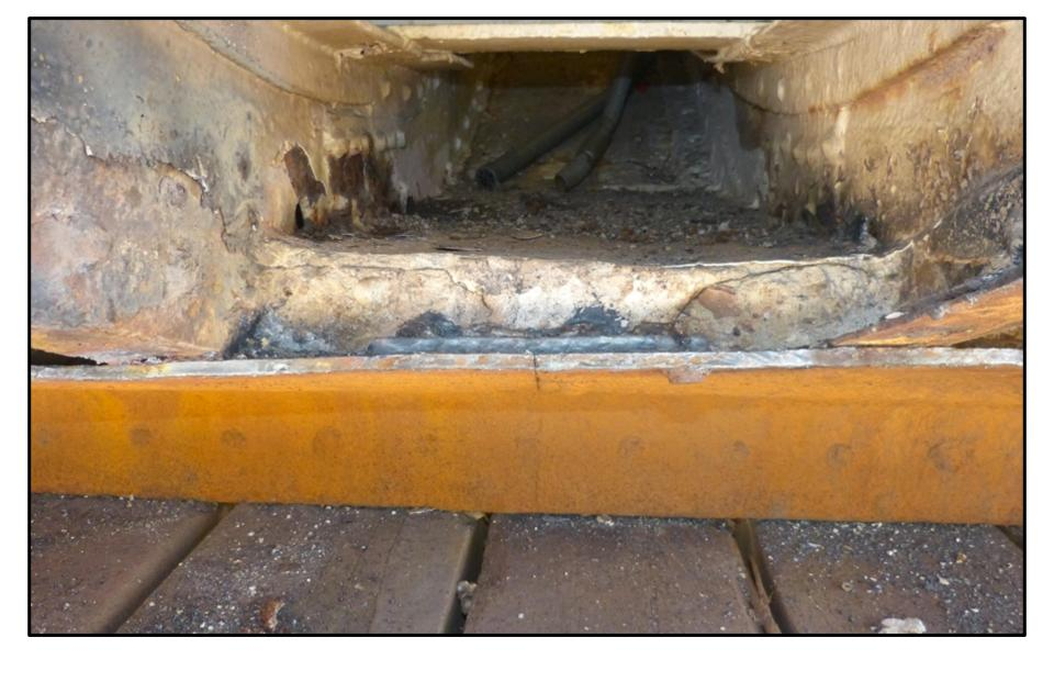
The cropped garboard plate showing the concrete and butt plate.
