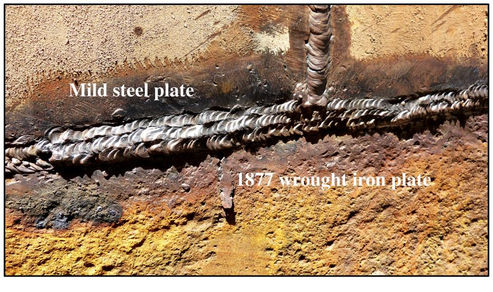
Example of welds. Special welding protocols were developed to weld modern steel to 1877 wrought iron.
