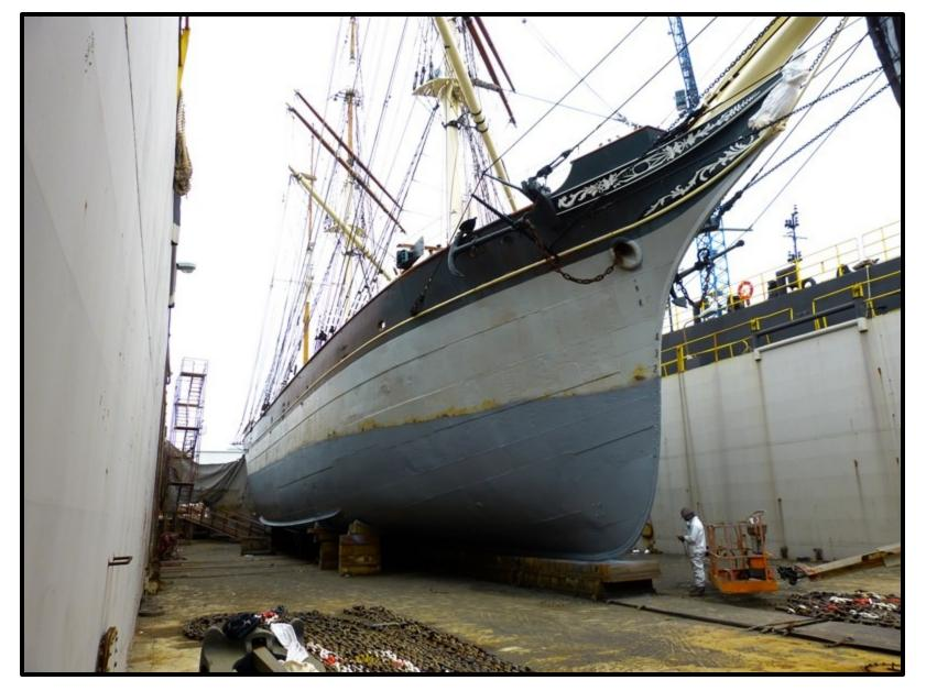
Ceramic coating applied at 150 degrees fahrenheit and 40 mils thick.
