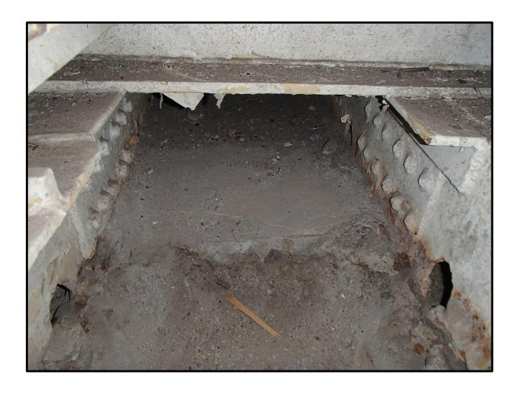
A typical frame bay and the concrete. The concrete served to allow water to drain through the limber holes in the frames and to serve as chafe protection from the abrasive action of salt water constantly washing over the iron plating - year after year.
