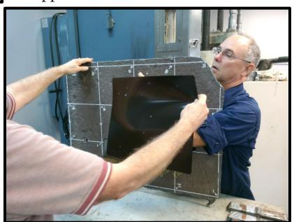
Test coupon of new steel plate welded to original 1877 iron plate sample to test weld integrity by pulling to destruction.
